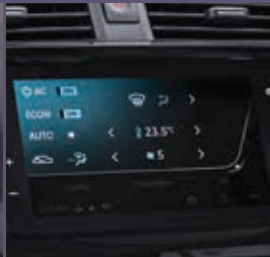
Automatic Temperature Control
