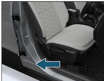
Chassis No. punching near driver seat
